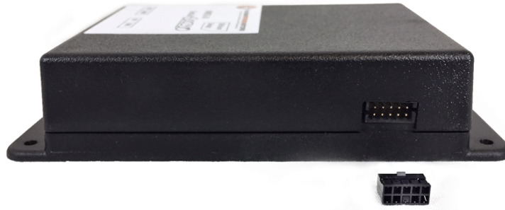
Figure 13 – BMSS Thermistor Connectors
