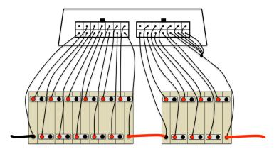
Pinout of cell connector
